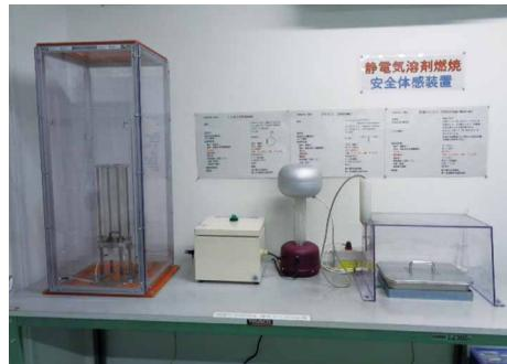
Electrostatic solvent combustion experience equipment
